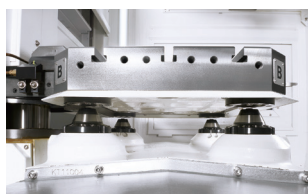
Pressurized Cones Repeatability 0.004 mm (0.00016")
