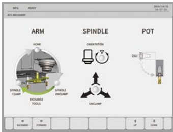
ATC RECOVERY function allows the operator to recover the tool changer.
