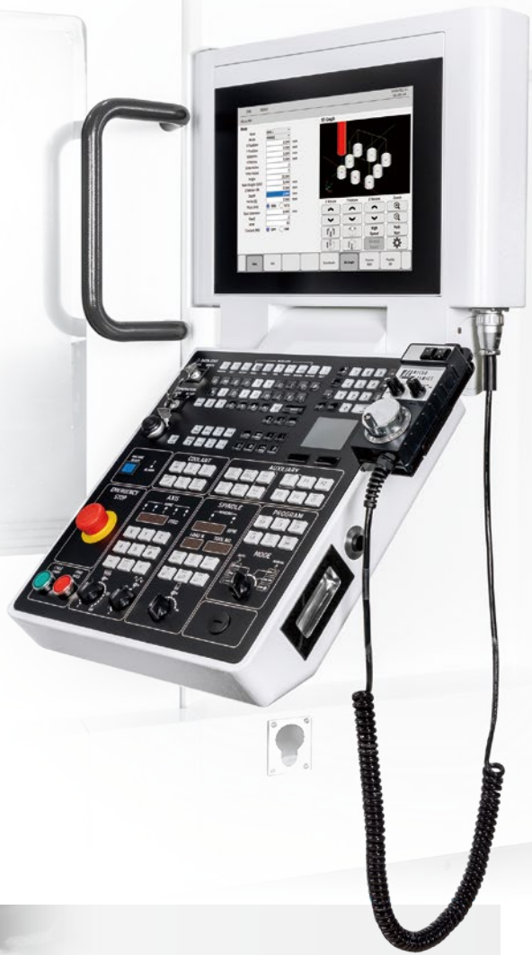
MICRO MILL® Conversational programming allows any operator to easily perform milling and drilling operations while creating G-Code and post to MDI or main memory.
