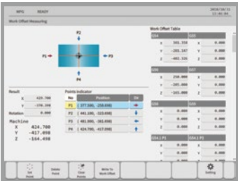
PART SETUP Fast and easy function for manually or automatically setup the part.
