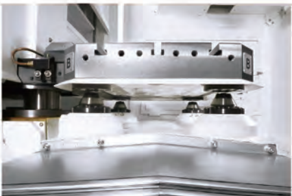
Pressurized cones Repeatability 0.004 mm
