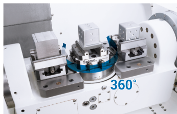
Rotary axis motion ranges
