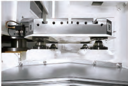
Pressurized cones Repeatability 0.00016"
