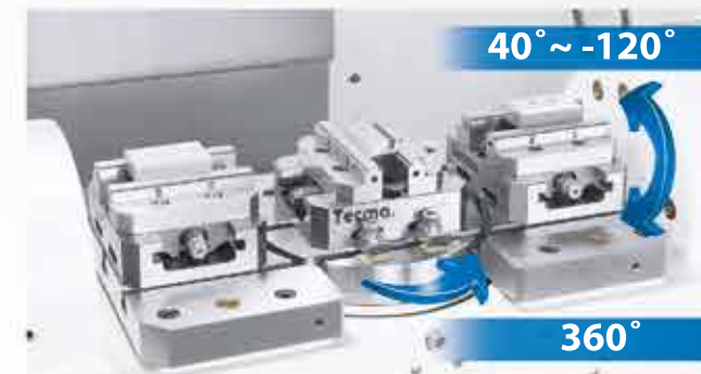
Titling axis and Rotary axis motion ranges.
