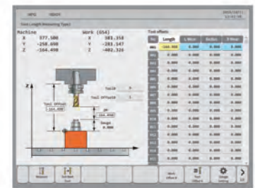
TOOL SETUP Fast and simple function for manually or automatically measure all the tools.
