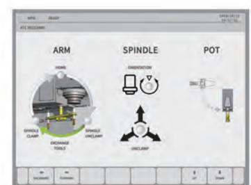
ATC RECOVERY function allows the operator to recover the tool changer.
