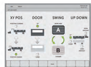
APC RECOVERY function allows the operator to recover the pallet changer.
