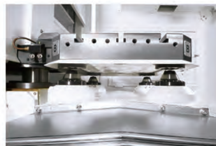
Pressurized cones Repeatability 0.00016"
