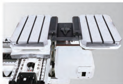
Servo driven pallet changer Switches tables in 8.5 sec
