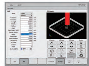
MICRO MILL® Conversational programming allows any operator to easily perform milling and drilling operations while creating G-Code and post to MDI or main memory.
