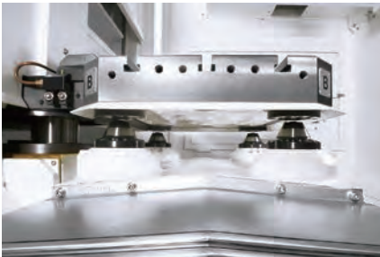
Pressurized cones Repeatability 0.004 mm
