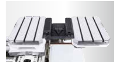
Dual pallet changer MEGA 20VAPC is designed for high production.
