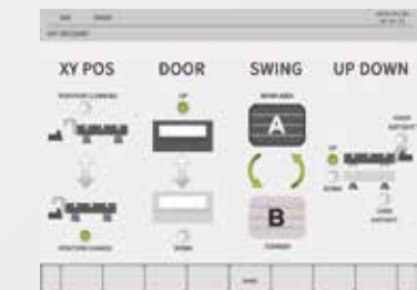
APC Recovery function allows the operator to recover the pallet changer.
